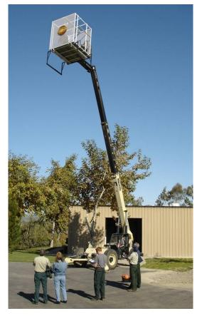
This Helicopter Simulator Cage holds four fire fighters at a time for rappelling training. The cage can be lifted up to 40' high by a specially designed forklift.
